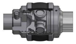
Joint protection: In the DHB e JHB series the joint rubber sleeve and clamp are protected from a particular device integrated inside the end of the auger feed screw. This characteristic is of considerable importance because it ensures the integrity of the joint in the case of pumping of abrasive substances or with solid blunt, without the needed to add expensive optional components.
